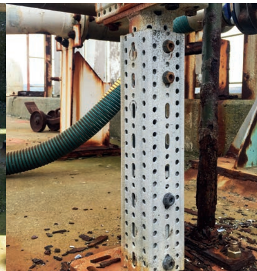
After 6 years of weathering – Offshore (CX)
